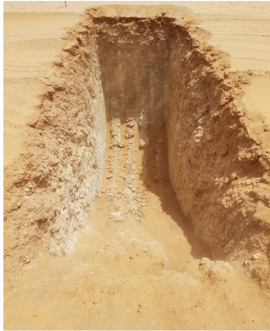
Figure 2. Bulk Sample Pit at the Tiris Uranium Project
