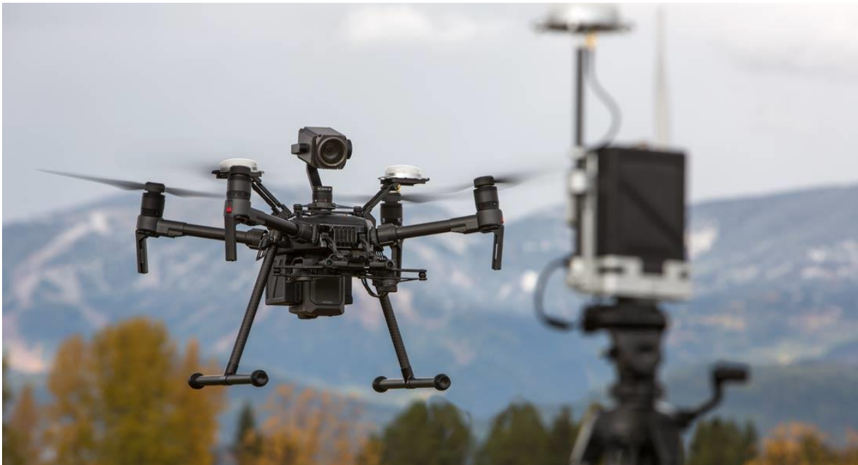
Figure Seven: M210 RTK UAV provides centimetre resolution aerial and survey capacity.
