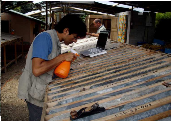
Cornerstone geologist Osman Poma logging drill core from drillhole CSD-13-001 from Alpala (Cascabel Project).
