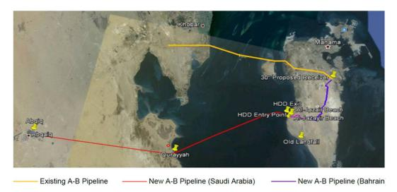
The front-end engineering design of the pipeline was completed in 2014 and separate contracts were awarded for the 43-kilometre long onshore Saudi Arabia stretch of the pipeline, the 41-kilometre offshore stretch and the 28-kilometre onshore Bahrain stretch. The new pipeline was completed and commissioned in October 2018, at which point decommissioning of the existing older pipeline commenced.
