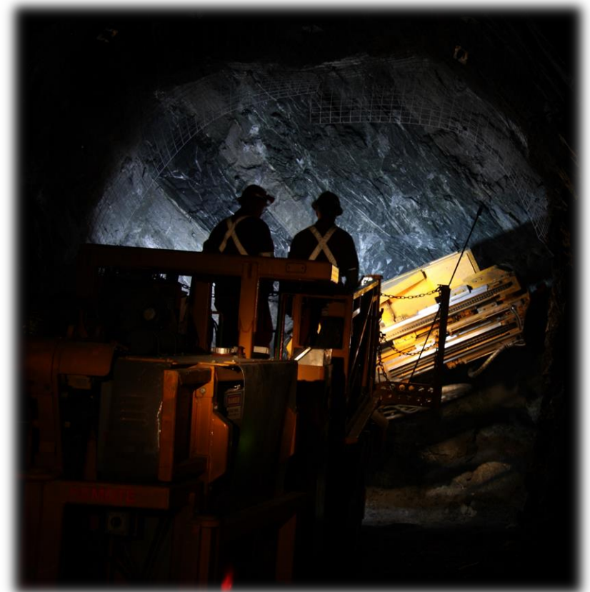
Bolting a development heading in the LFZ
