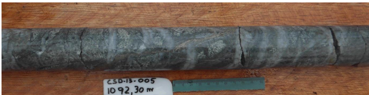
Hole CSD-13-005 (1092.3m) - Intense quartz and quartz-magnetite stockwork veining in chlorite-sericite altered hornblende-diorite and cross-cut by a pyrite-chalcopyrite vein.
