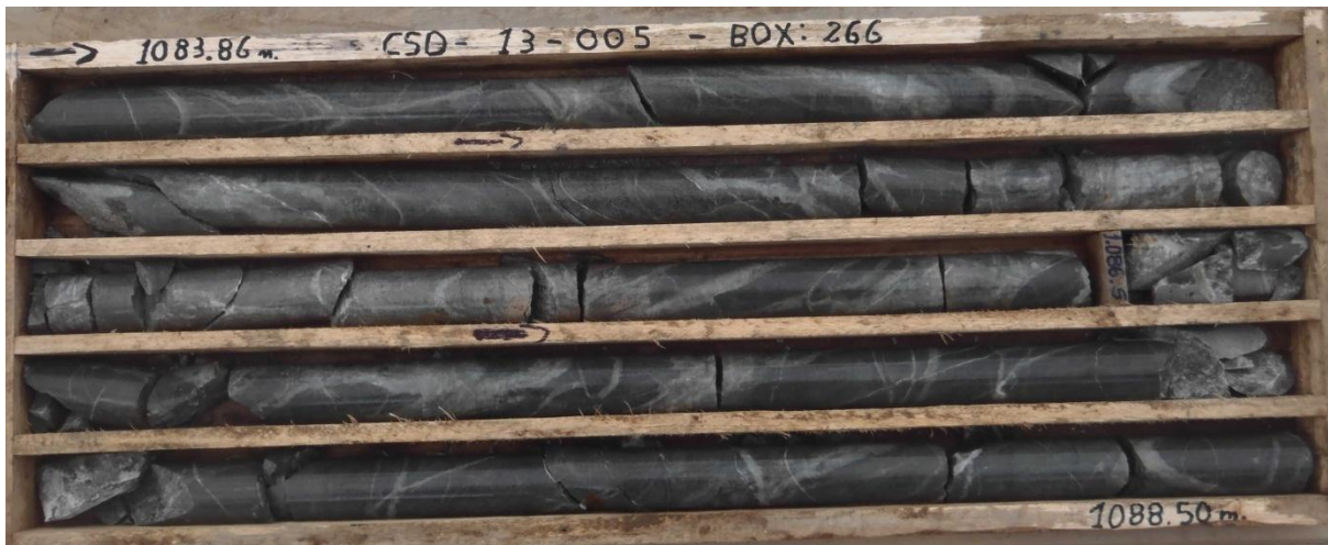
Hole CSD-13-005 (1083.86m to 1088.50m) - Intense quartz stockwork veining (approximately 20 veins per metre) in magnetite-bearing and potassic-altered diorite.
