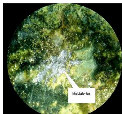
Photo 4.4: Drillhole BAI-5 at 58.5m
