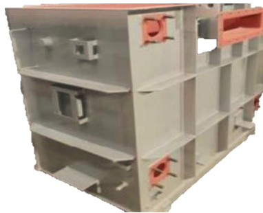
Transformer Cover (HR Grade: S355MC 5-6mm, impact guarantee at -48°C)
