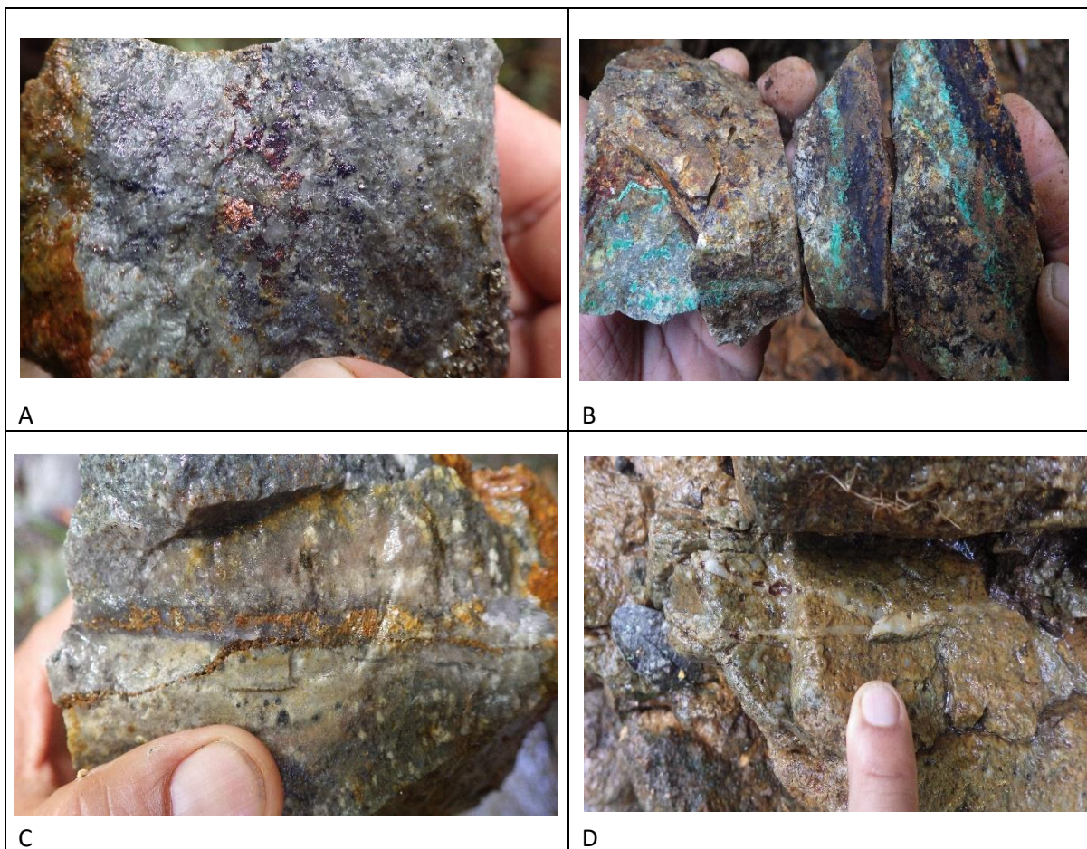
Photos 4: Target 6 at La Hueca - Diorite with strong chlorite epidote prophylic alteration. Chalcopyrite - 0.5 to 3.5%, malachite ~ 0.8%, chalcocite ~ 1% and bornite ~ 0.1%.
