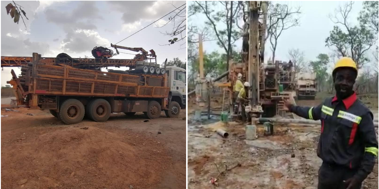
Figure 1: RC drill rig arriving on site and drilling underway with IronRidge field team supervising.
