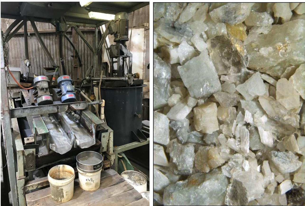
Figure 1 | DMS100 cyclone metallurgical test-work equipment at Nagrom, Perth (left) and SG2.9 Underflow high-grade spodumene concentrate crushed and screened at P100 6.3mm + 0.5mm (right; field of view approx. 4cm across).
