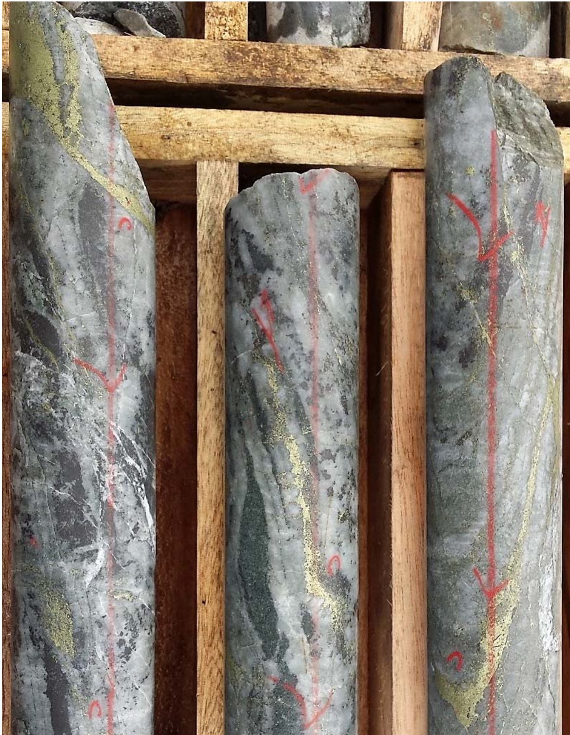
Figure 2: Drill core samples from CSD-15-011 from 996.6m depth showing intense porphyry stockwork mineralisation encountered. The multi-phase nature of mineralisation, evident here as early magnetite-chalcopyrite-bornite quartz veins, overprinted by massive chalcopyrite veinlets, has produced very high grade results in previous drill holes.
