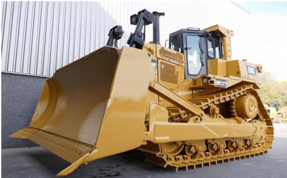
Figure 3: D9 Caterpillar dozer ready to be deployed and added to the mining fleet at Dundas. The 49 tons D9 dozer will also be used in the production of the ilmenite-bearing sand bulk-sample, related infrastructure development and ship loading operation at Dundas this year.
