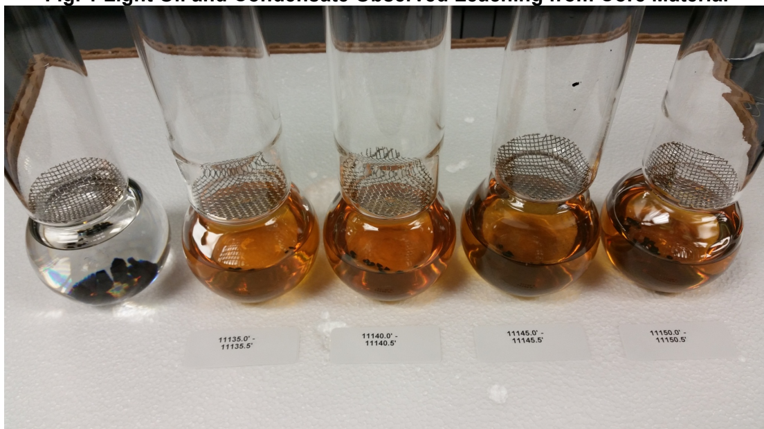
Fig. 1 Light Oil and Condensate Observed Leaching from Core Material
