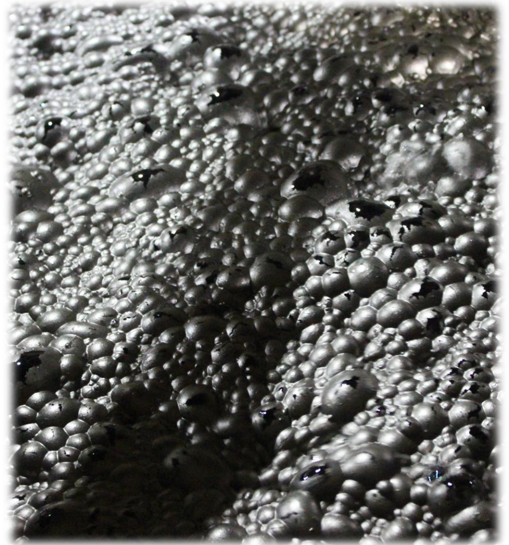
Copper concentrate in the final stages of production at Nugget Pond
