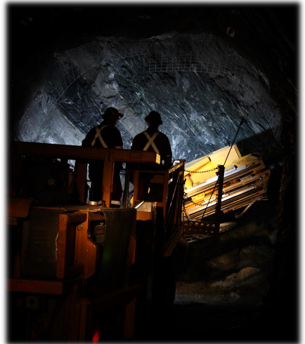
Mechanical bolter adding ground support in the LFZ ramp
