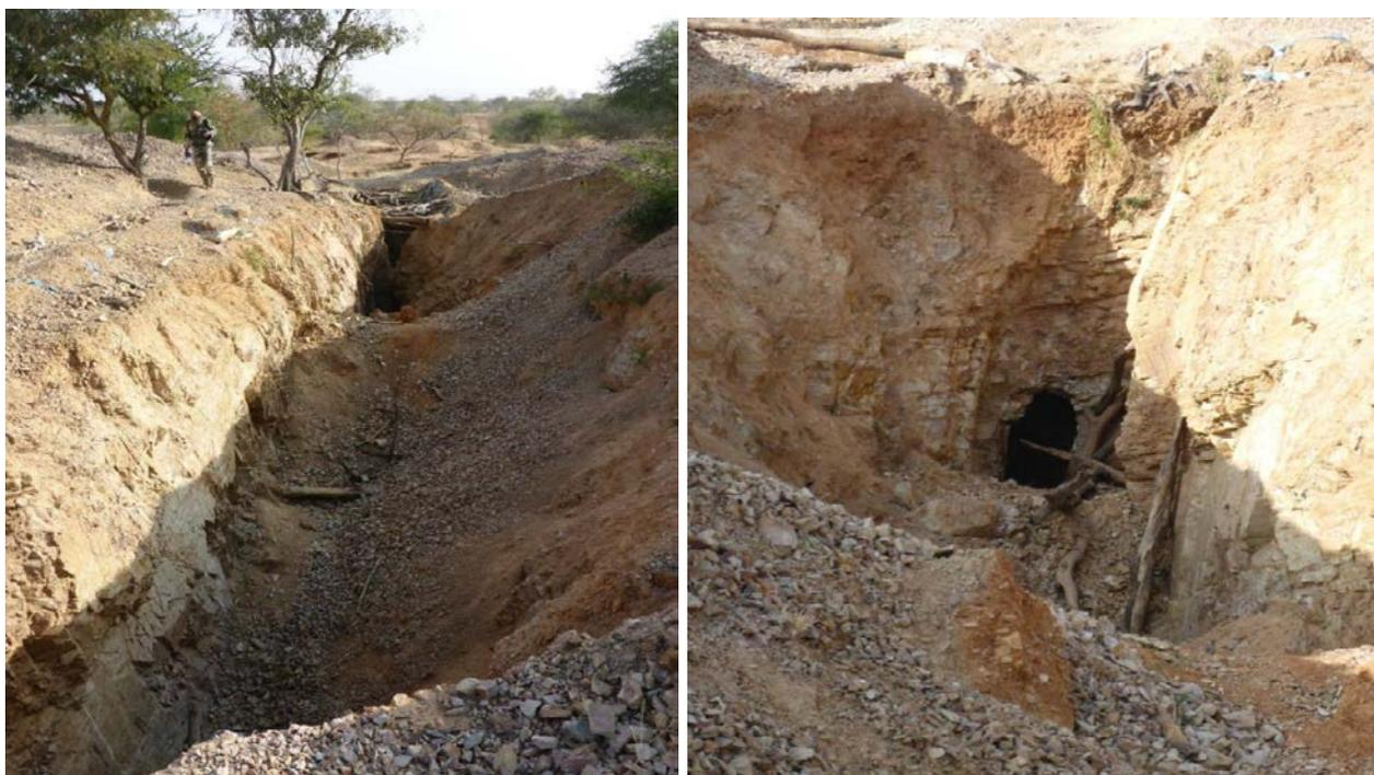
**Figure 3** | Camp 1 artisanal workings exposing mineralised veins in rock face
