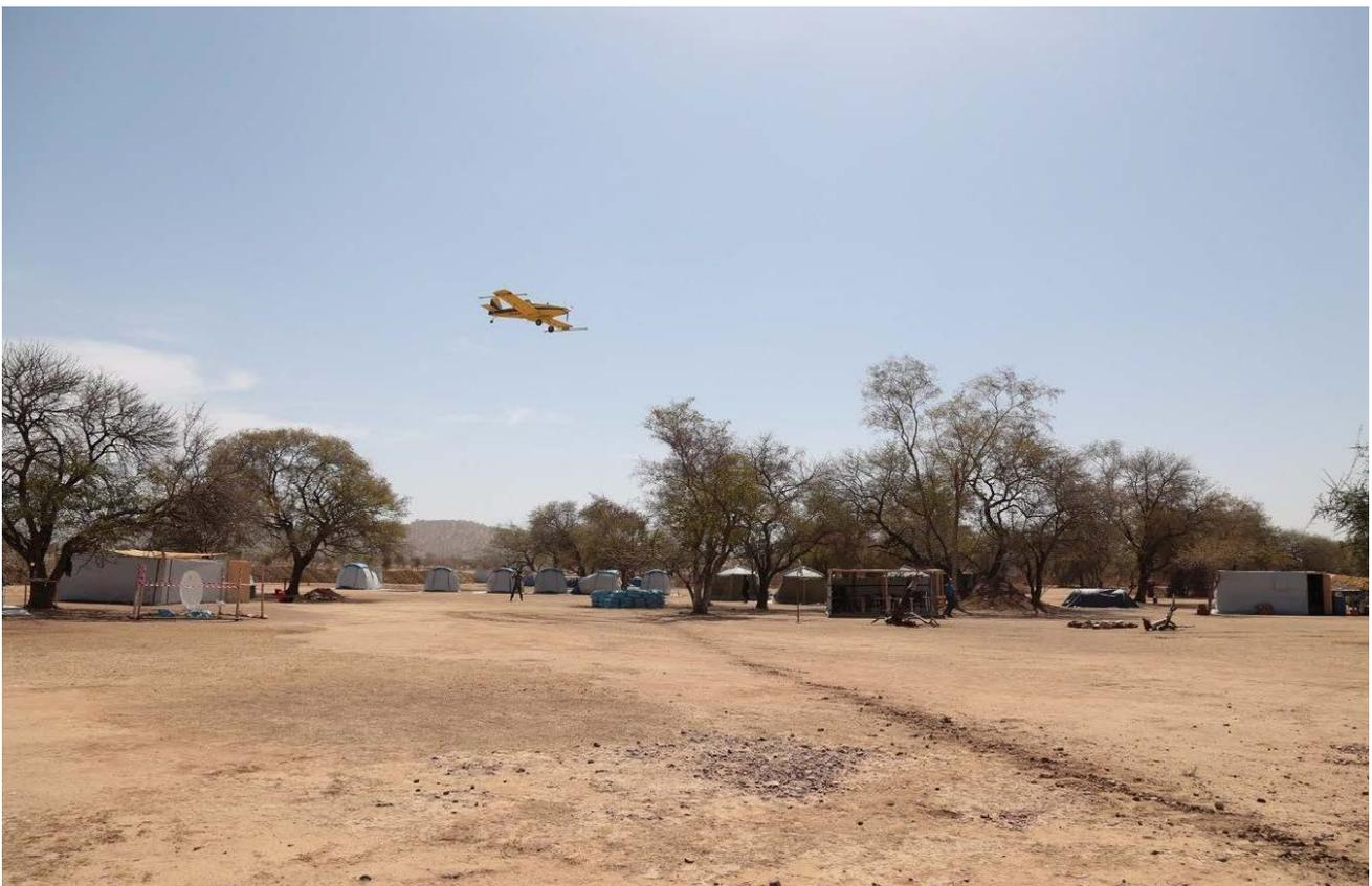
**Figure 5** | Xcalibur aircraft flying aeromagnetics survey over Dorothe Main camp
