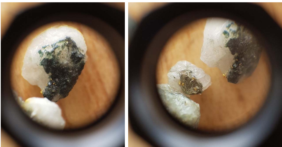
Figure 4: Visible gold observed through a hand lens in drill cuttings from hole ZARC0019 between 82m to 83m depth downhole (field of view approximately 1cm across).
