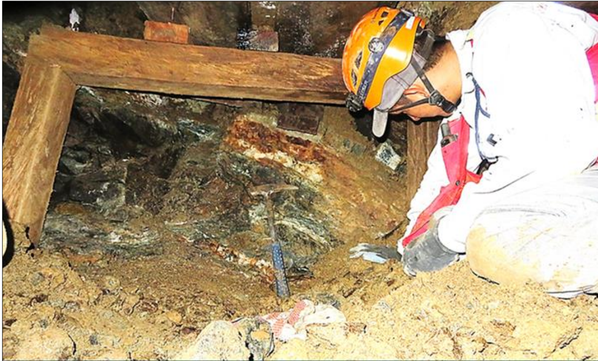
Photo 4: Examples of polymetallic gold-telluride veins at existing underground artisanal workings at the Cielito Vein System.
