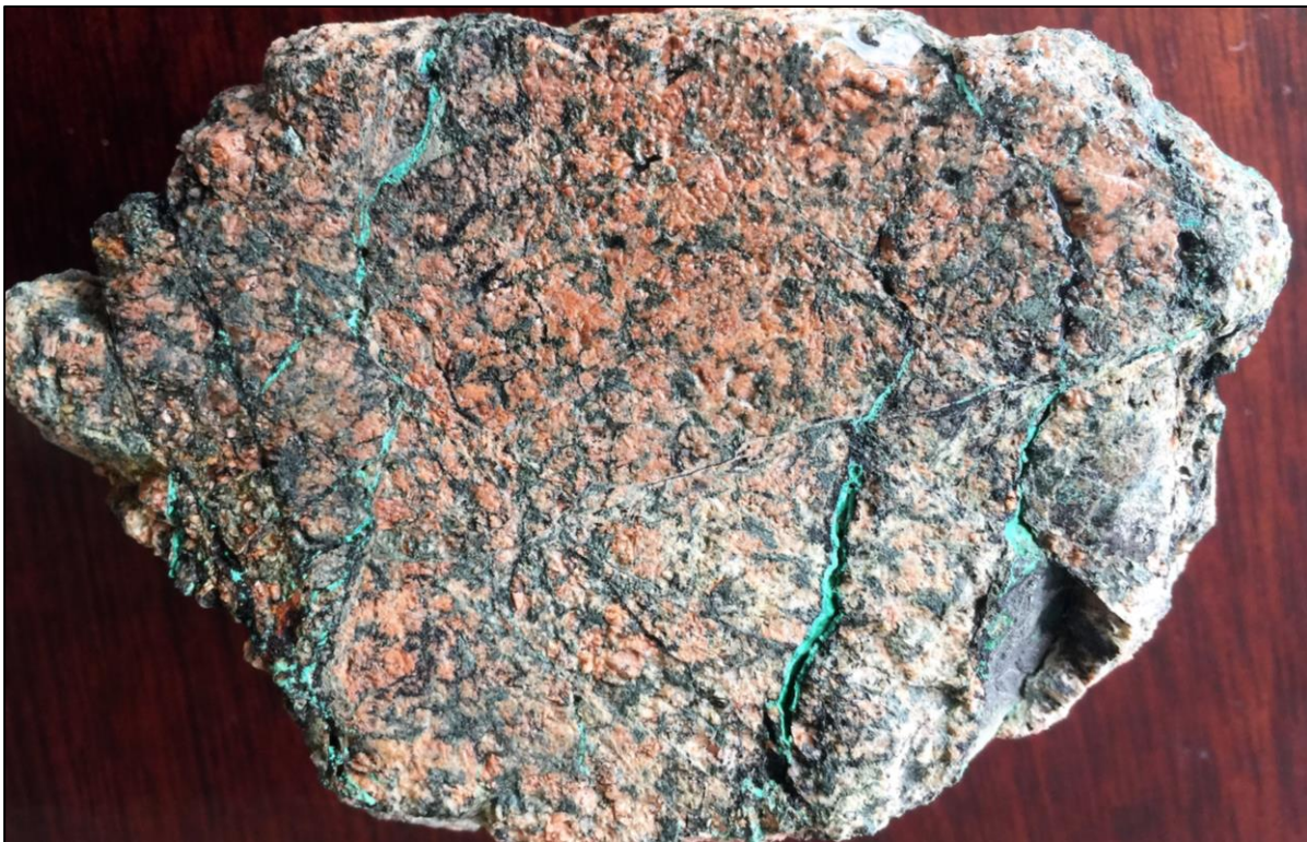
Figure 3: Potassic altered diorite outcrop from Porvenir project exhibiting disseminated chalcopyrite and strong secondary Cu mineralization, as indicated by fractures filled by malachite (green mineral).
