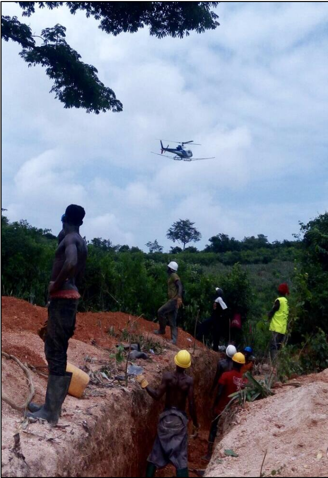
Figure 2 | New Resolution Geophysics (NRG) helicopter with geophysical equipment taking off from Cape Coast base and (right) trenching underway at the Ewoyaa prospect with light coloured spodumene bearing pegmatite in the trench.
