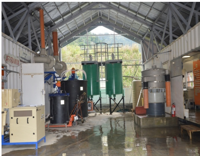
Image 1: On site operational ASTER™ & Biox® (left) and Flotation (right) minilab
