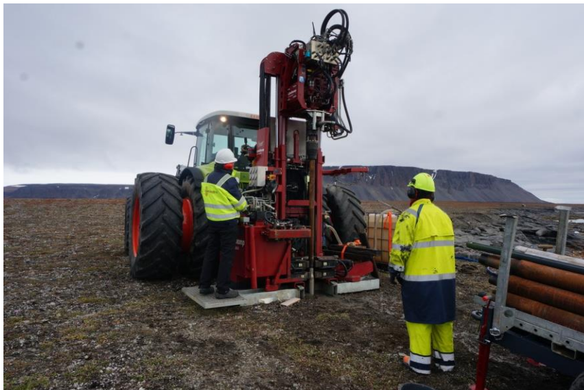
Figure 2: White Eagle’s tractor-mounted Sonic Drill on the coastal plain with the Dundas Mountains in the background.
