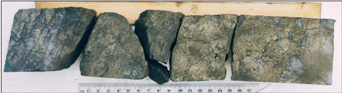
Figure 2: Split section of drill core from hole FR-DD-22-UG-183 grading 75.9 g/t Au and 90 g/t Ag over 0.26 metres.
