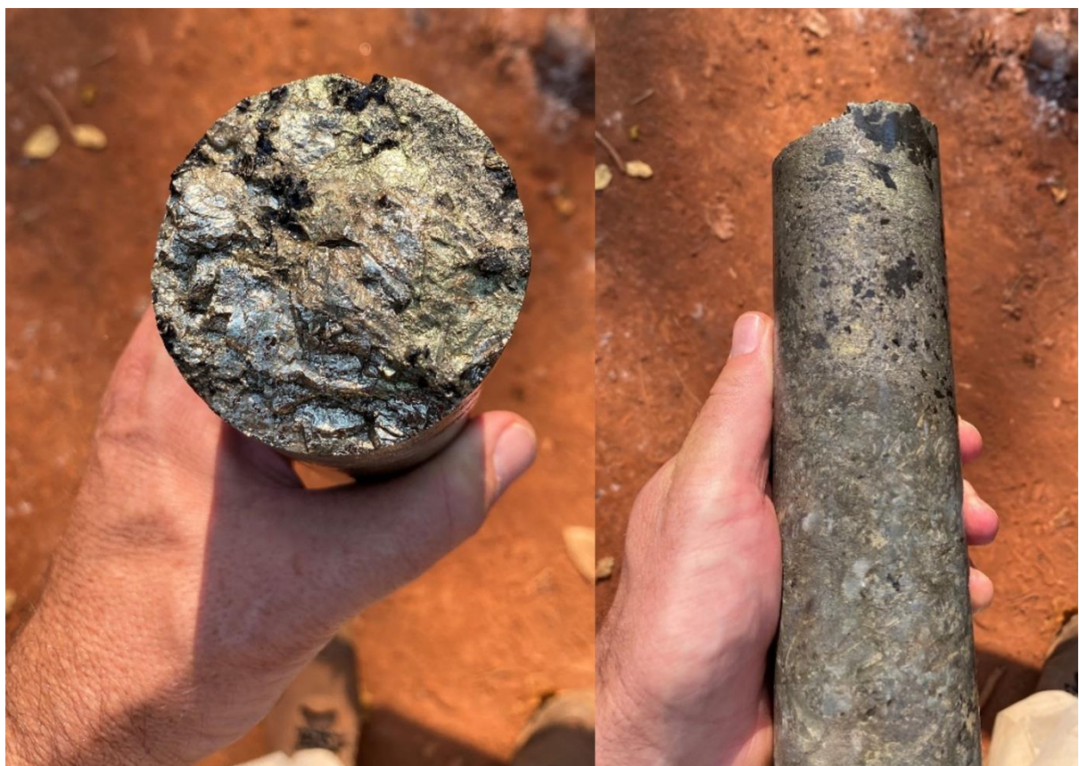
Fig 2. Diamond drill core of massive sulphide mineralisation.
