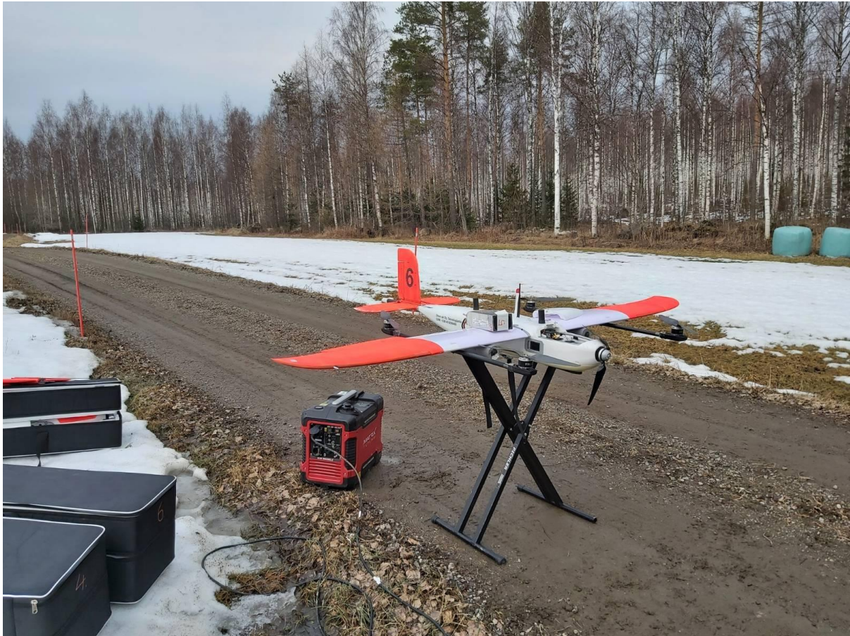
Figure 2 The Vertical take-off fixed-wing UAV from Radai Ltd used for the three-component magnetic survey conducted in mid-April over an area south-east of the past-producing Laukunkangas Ni-Cu-Co mine within the Enonkoski Project area. The survey was done to refine drill targets as well as to test the acquisition method and data quality in considerations for a possible larger survey.
