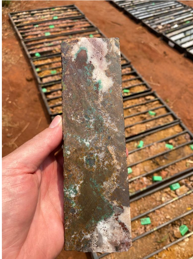
Figure 1. Half core of high grade copper mineralisation, mostly chalcocite with lesser malachite
