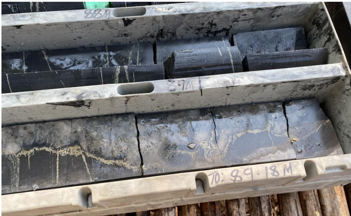
Figure 3. Carbonaceous shale intruded by a vein, realigning the sulphides to the margin of the vein
