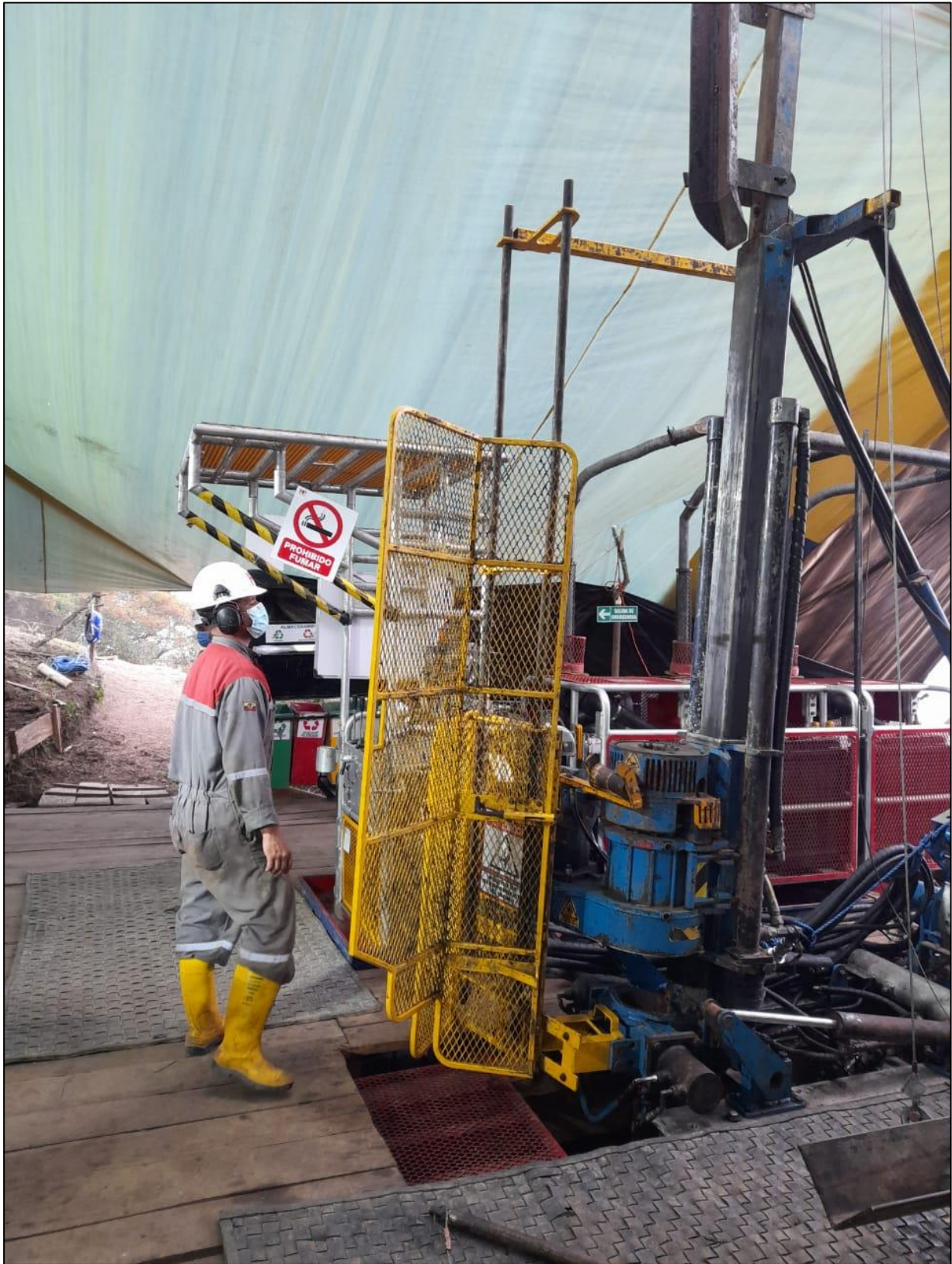
Figure 4: Drill hole 1 (RDH-21-001) underway at 90m depth, drilling towards a planned depth of 1,500m utilising customised man-portable drill rig.
