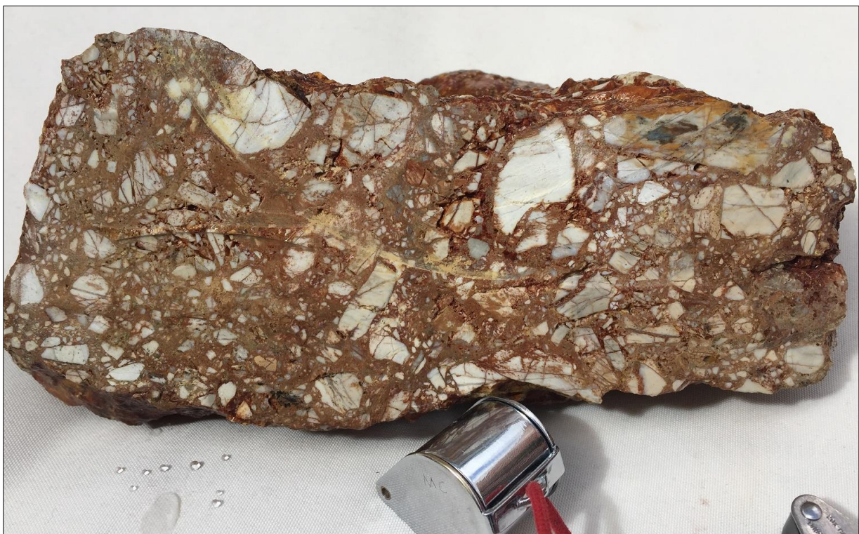
Figure 9: Example of gold bearing hydrothermal breccia containing clay altered lithocap fragments. This sample returned an assay result of 1.0g/t Au.
