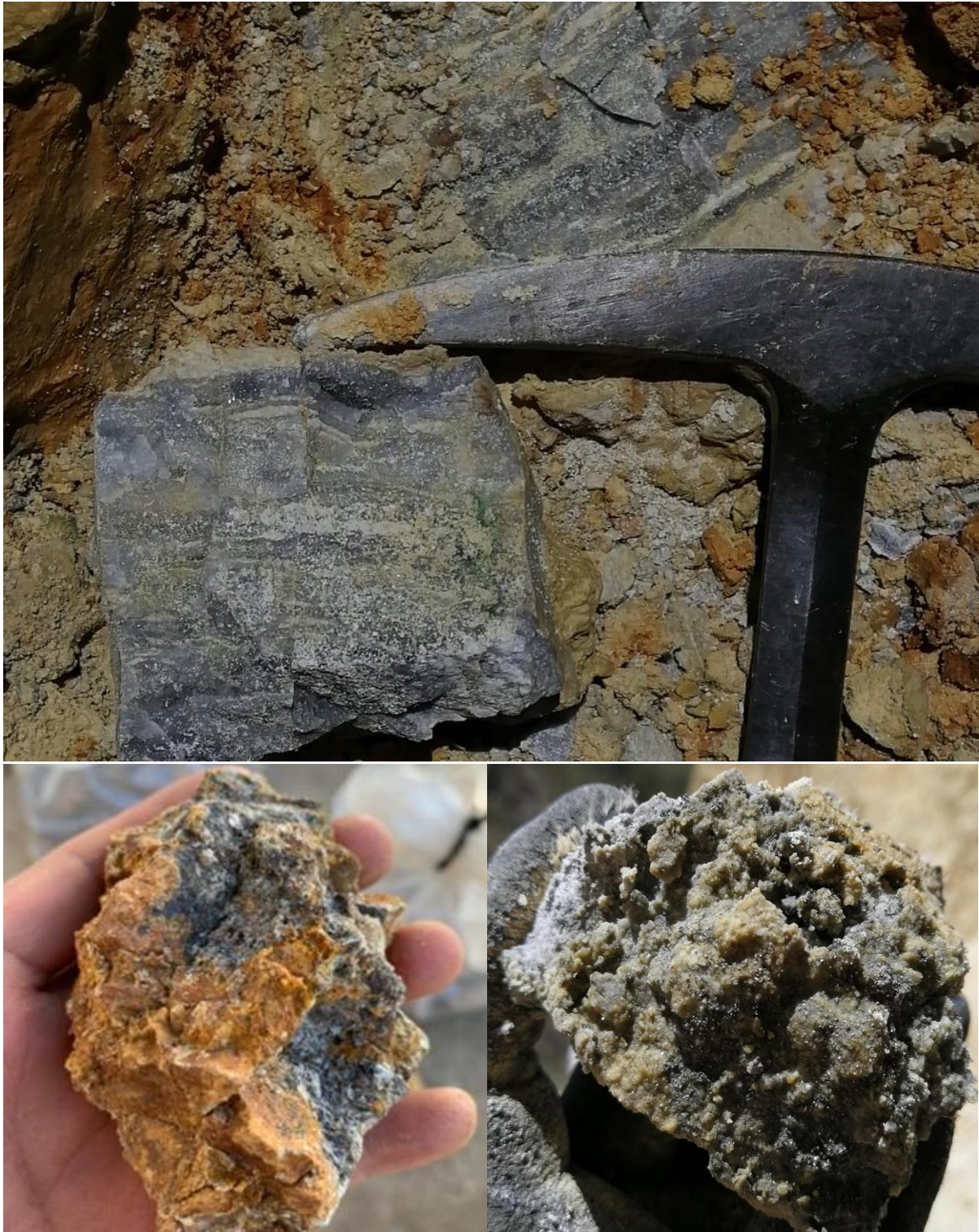
Figure 10: Strongly altered rocks from the upper Varela lithocap, containing B-type porphyry veins and visible trace chalcopyrite and molybdenite mineralisation. Assay results pending.
