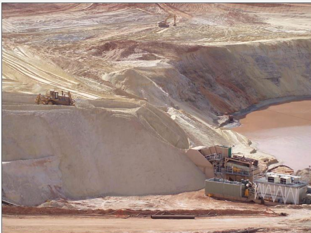
Figure 5: Example of dry mining using dozer trap
