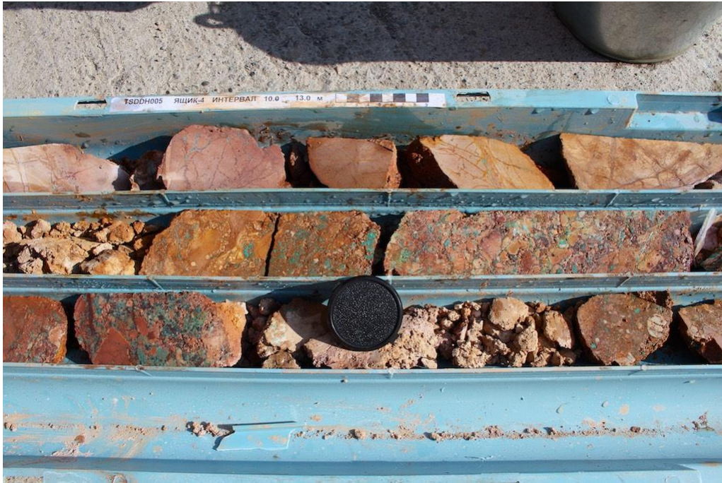
Image 1: Drill core from 10.00-13.00 metres showing high grade copper mineralisation
