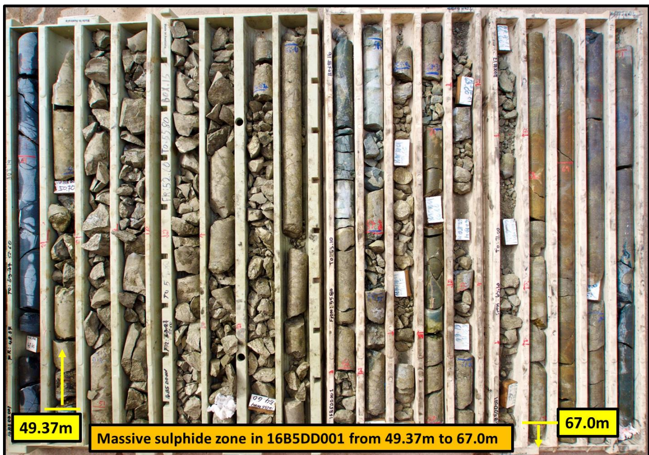
Figure 4. Diamond drill core from 16B5DD001 showing the massive sulphide zone
