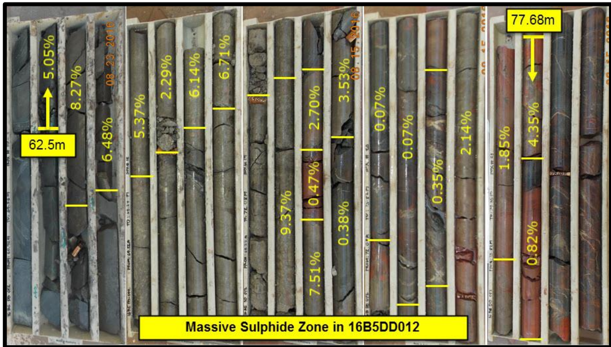
Figure 2. Diamond drill core from 16B5DD012 showing the massive sulphide zone
