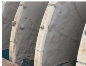
Figure 2 – Flotation product undergoing filtration for reduction of moisture content to <5%
