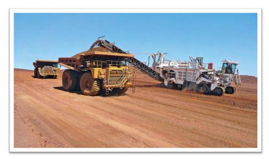
Figure 5: Surface mining method (FMG, Pilbara WA) from the ground straight into a truck
