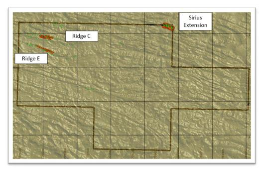
Figure 2: Tenement boundary and target location. Drill collars shown in green, and the optimised pits shown in red
