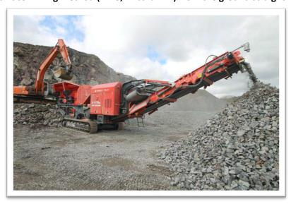
Figure 6: Example of a mobile screening and crushing plant
