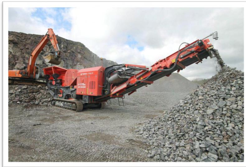
**Figure 6: Example of a mobile screening and crushing plant**
