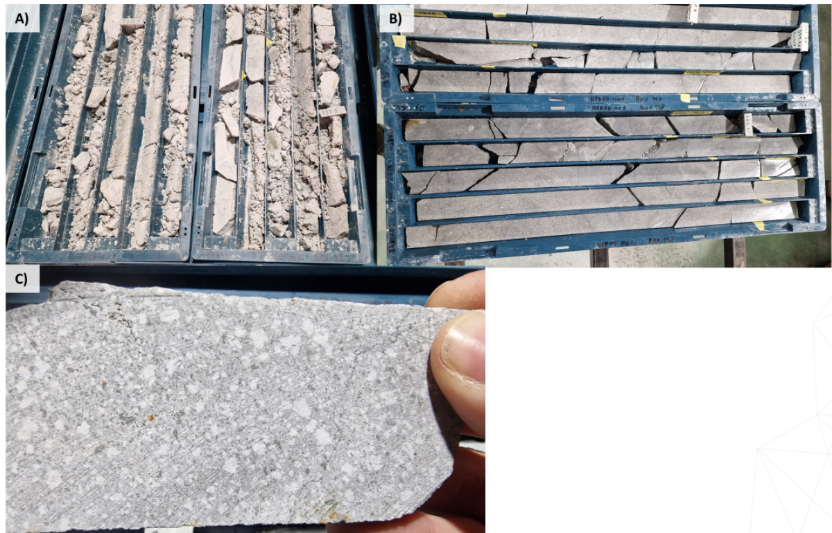
Figure 3: A) Towards the end of hole HERDD001, bleached, broken, and intensely altered porphyritic andesite is observed. B) weak-to-moderate potassic altered drill core in HERDD001 at approximately 550m. C) Porphyritic andesite with moderate alteration with kaolinite in HERDD002 at approximately 740m.
