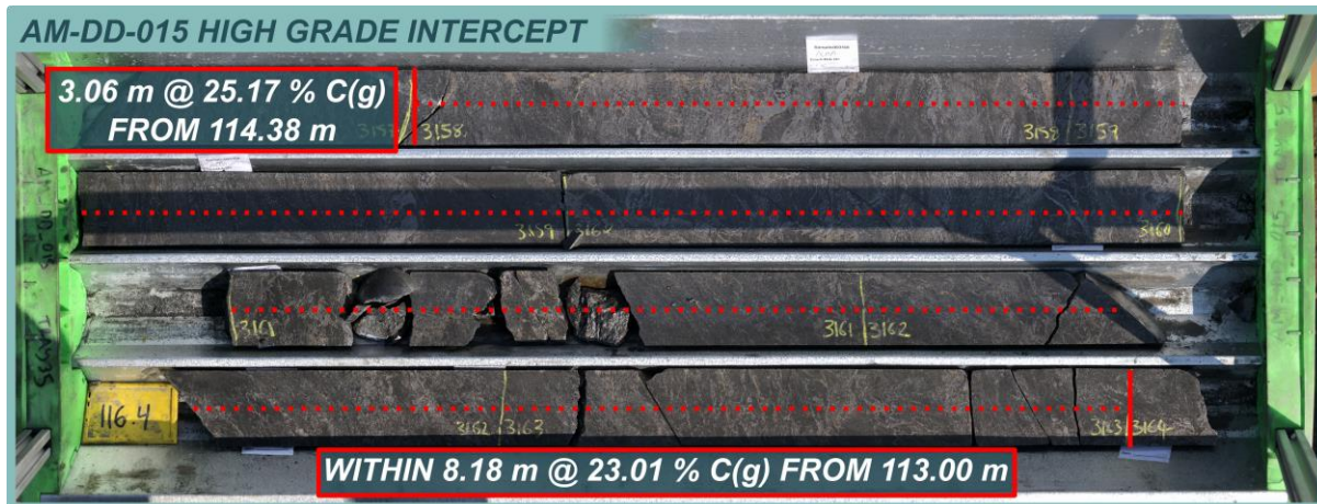
Figure 9. High-grade LGL intercept in AM-DD-015. This lies within the 8.18 m intersection (see Table 1).
