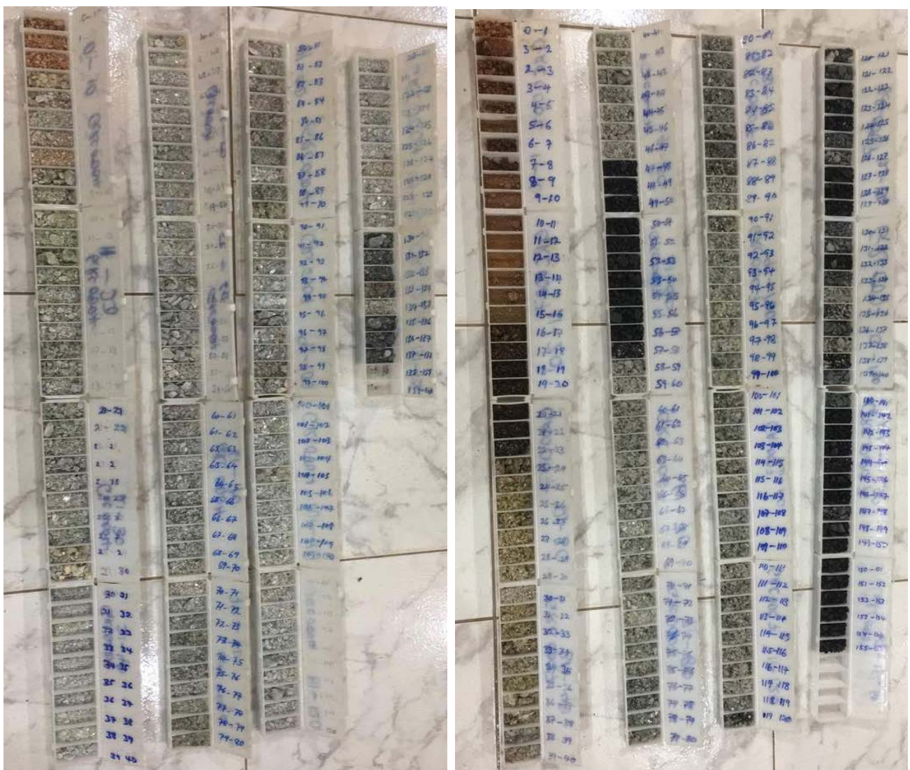
Figure 1 | RC chip trays for drill hole GRC0004 (Left); 130m continuous intersection of visible pegmatite (light coloured RC drill chips) from surface and drill hole GRC0007 (right); 24m and 62m intersections of visible pegmatite (down hole meterage marked on trays) – Assays pending.
