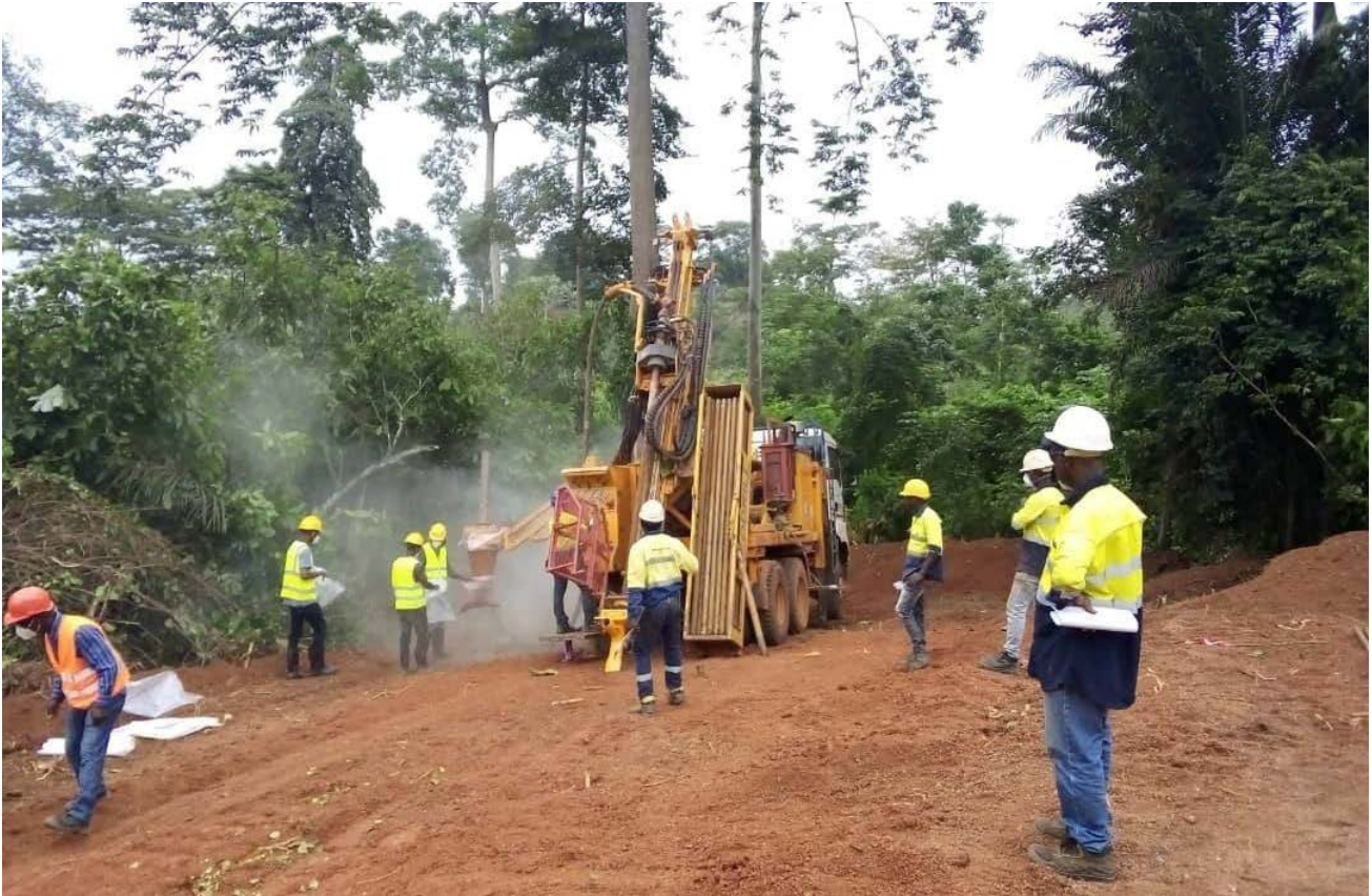
Figure 1: Air-Core rig currently drilling at the Ebilassokro target.
