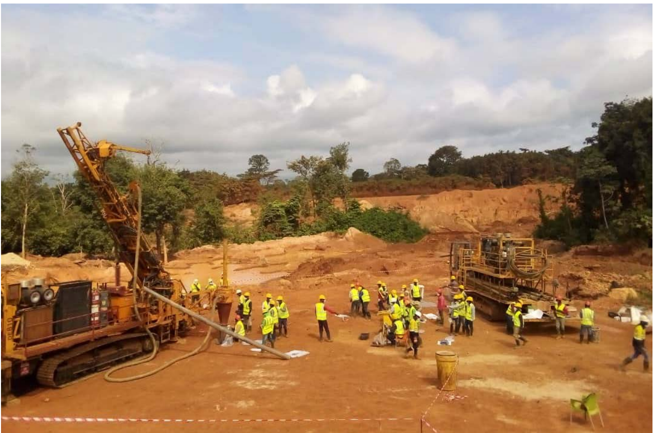
Figure 2: First of two reverse circulation drill rigs currently drilling at the Ehuasso Main target.
