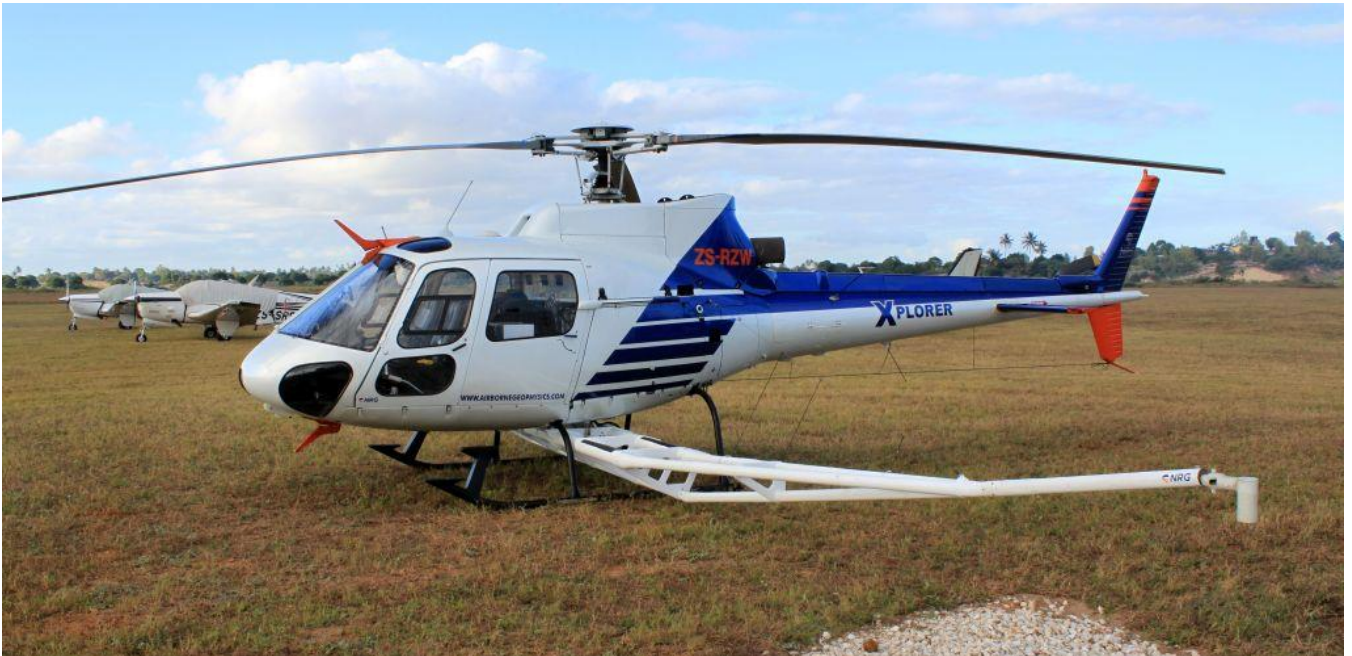
Figure 1. NRG (New Resolution Geophysics) heliborne AMAG / RAD platform onsite at Jangamo Project
