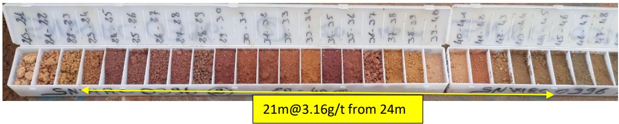
SW photo of sample for the 8 m at 7.04 g/t from 23 m (SNWRC0364)
