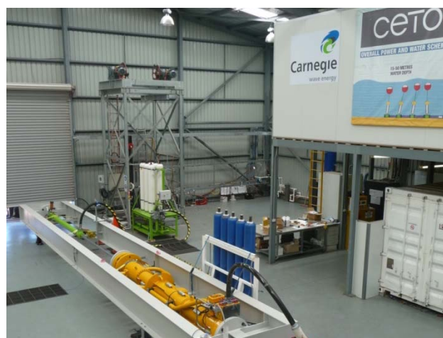
CETO onshore pump and hydraulic test rig at Carnegie's Fremantle Test Facility
