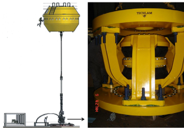
Pump to Foundation Attachment
