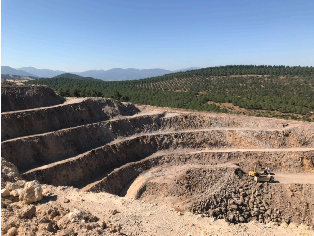
Figure 2: Derya pit, with pushbacks underway on the southern wall, extending to the east. Some of the best grades ever encountered at Derya are going to be accessed following the completion of this pushback.
