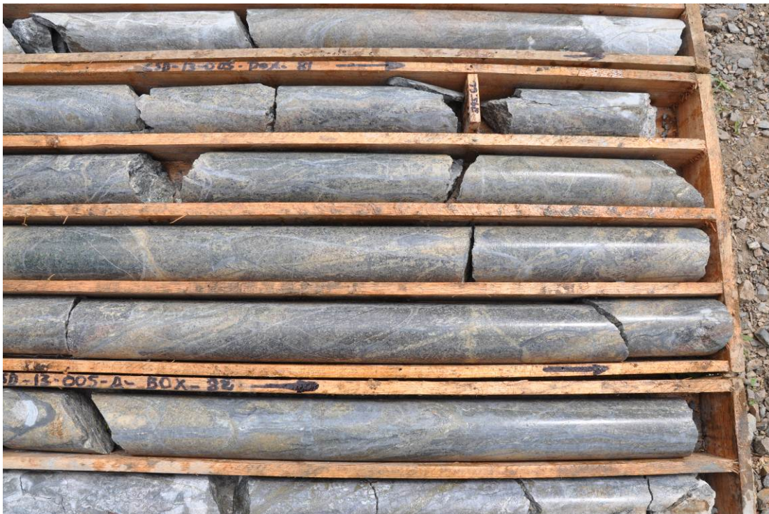
Figure 9 – Drill core from hole CSD-11-005 from the Alpala prospect (around 295-298.55m depth), showing sheeted and cross-cutting sets of porphyry quartz-chalcopyrite veins in a strongly potassic-altered diorite protolith (the potassic alteration has a phyllic alteration overprint).
