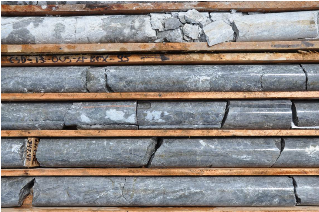
Figure 10 – Drill core from hole CSD-11-005 from the Alpala prospect (around 347.47m depth). Intensely sheeted porphyry-related quartz ‘B-veins’ with very fine grained disseminated bornite mineralisation and coarse chalcopyrite mineralisation in cross-cutting albite-chalcopyrite veins.
