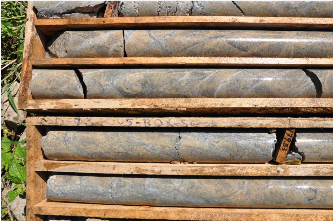
Figure 8 – Drill core from hole CSD-11-005 from the Alpala prospect (around 179.03m depth), showing typical high density of mineralised cross-cutting quartz vein networks within potassic-altered diorite intrusion which is affected by retrograde phyllic overprint (defined by the tan-coloured sericite alteration and the conversion of magnetite to hematite).
