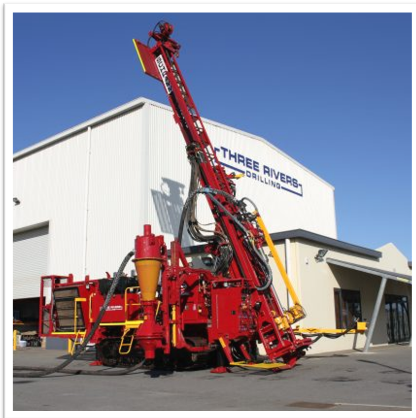
Figure 2: T450 Reverse Circulation (RC) drill machine, Three Rivers Drilling, WA.
