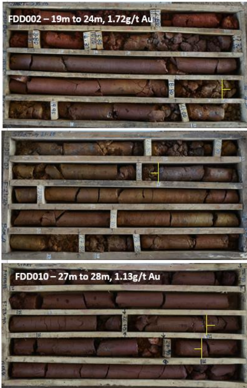
Figure 2: Drill core and mineralised intersections from holes FDD002 and FDD010
