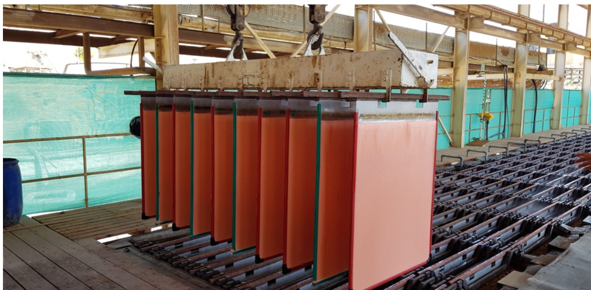
Figure 2: High purity copper cathode production following SX-EW processing at Skouriotissa. The final product at Apliki will be the same.
