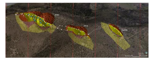
**Figure 1:** Three-dimensional model of the Kizilcukur vein system looking due north, showing the modelled ore zones within Whittle optimised pit-shells (based on the 2016 resource) and current drilling. Historical drill hole collars are shown as white dots, while the 2019 in-fill drilling is shown with blue dots.
