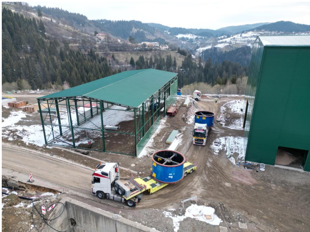
Figure 7: Oversized delivery of mill at VPP
