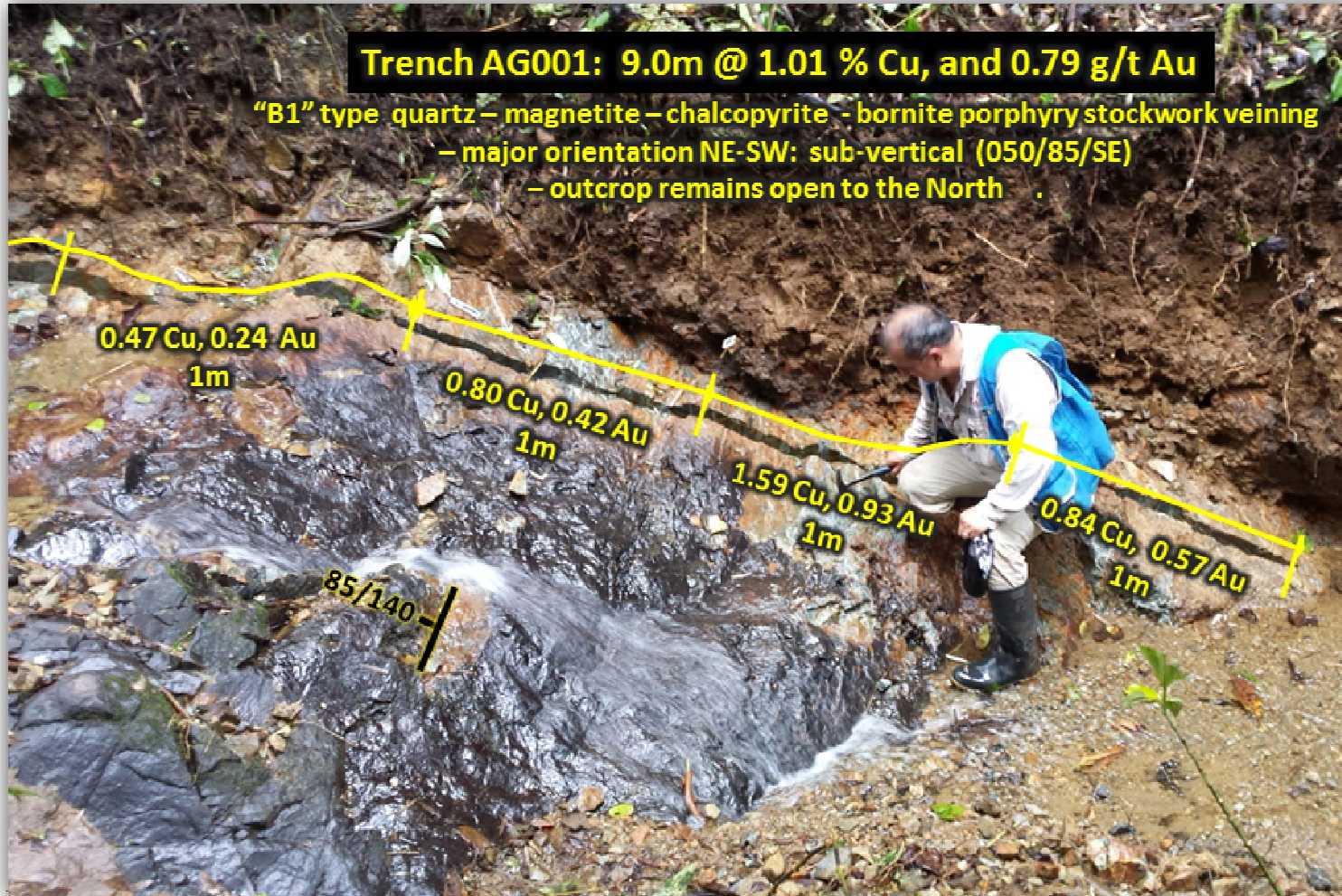
Figure 3: The northern end of Trench AG001 showing rock-saw channel results over mineralised diorite porphyry.
