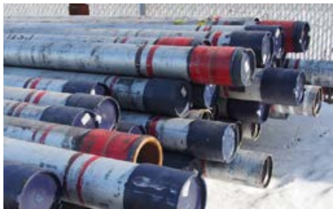
VACUUM INSULATED TUBING FOR STEAM ASSISTED EXTRACTION IN THE CANADIAN OIL SANDS.
