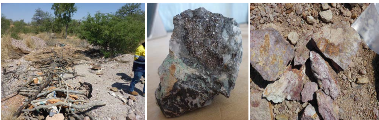
Figure 3 | Left: New artisanal working (covered with sticks and now abandoned), mined to a 10m vertical depth. Centre: High-grade sample (approx. 5cm width) from workings with extensive visible galena and secondary copper minerals. Right: Extensive jarosite and pyrite in wallrock alteration around newly exposed artisanal workings
